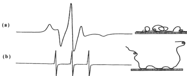
Figure 2. Representative ESR spectra for a nitroxide-labeled polymer and the corresponding suggested orientation/mobility.
